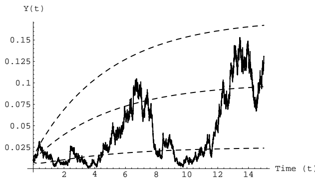
Figure 14.4: SAMPLE PATH OF SQUARE-ROOT PROCESS. Depicted is a sample path of the square-root process dY = 0.2(0.1 - Y)dt + 0.15\sqrt{Y}dW with the initial condition Y(0) = 0.01 . The envelope is for one standard deviation around the mean 0.01e^{-0.2t} + 0.1(1 - e^{-0.2t}) .
