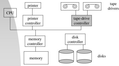
Device controllers: synchronize and manage access to devices.
