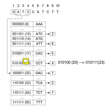
Figure 12: A hash table for GATCCATCTT under a weight three model 11\*1.
