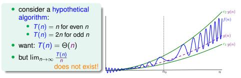
fixed (formal) definition ver. 1: for asymptotically non-negative f(n) and g(n),  $f(n) = \Theta(g(n))$  if and only if there exists positive  $(n_0, c_1, c_2)$ such that  $c_1g(n) \le f(n) \le c_2g(n)$  for all  $n \ge n_0$
