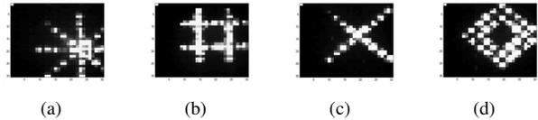
Figure 3. The 30x30 images captured by the mouse sensor when different patterns are used (a) Star-shaped (b) Sharp-shaped (c) Cross-shaped (d) Double-diamond-shaped with 2 pixel spacing
