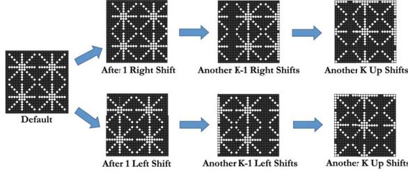
Figure 4. Simulation of the moving patterns of binary movement shift keying
