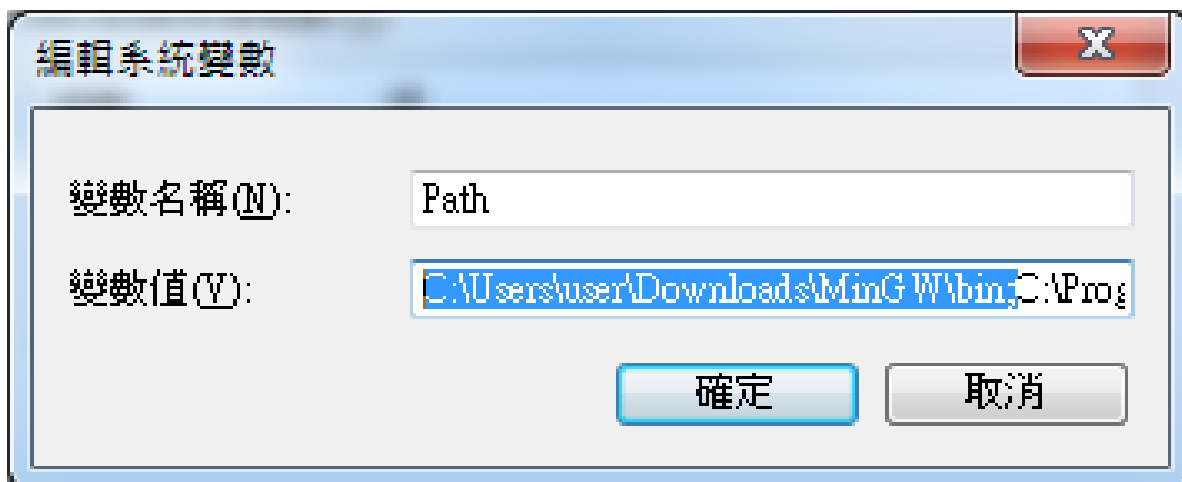
Figure 8: Add the previously copied path of bin/, followed with a semicolon(;), to the left side. Confirm many times.
