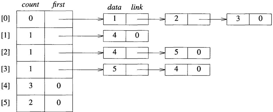
**Figure 6.39:** Internal representation used by topological sorting algorithm
