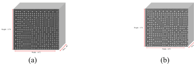
Fig. 1. (a) The 3D PCB model reconstructed with 128 different angles of 2D X-rays images. (b) The 3D PCB model reconstructed with 16 different angles of 2D X-rays images.
