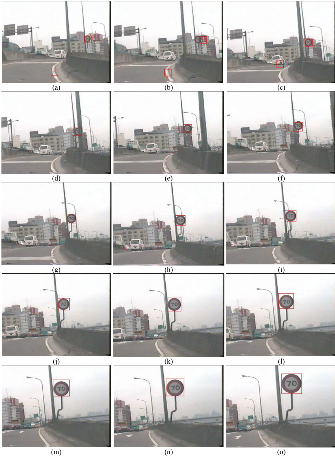
Figure 5: The experimental results with video sequence S_l . The first fifteen frames of this sequence are shown in (a) to (o). The size of each image is 320 \times 240 pixels and the time between two successive images is 0.2 second.
