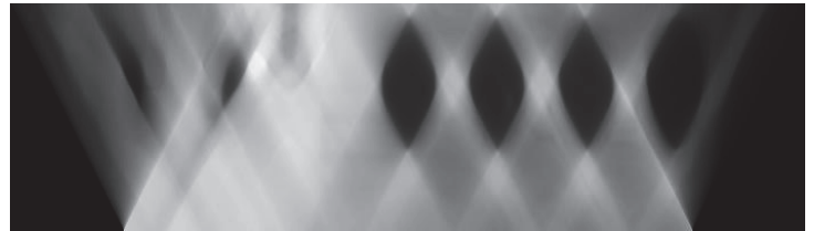
Fig. 29 The above is the image we reconstruct with x=350 . We can see that the shape of solid ball in the image we reconstructed is not ball but rhombus.
