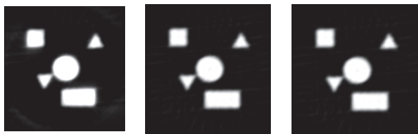
Fig. 3 Reconstructed from sinogram using 32 projections and addition algebraic reconstruction technique with (a) 1, (b) 100, (c) 500 iterations.
