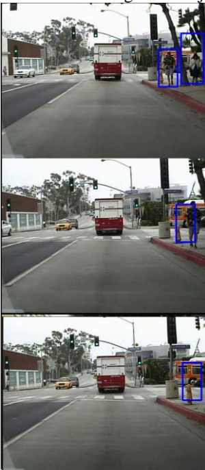
Fig. 27 Sample 3 of wrong tracking caused by approaching pedestrian and much larger block size.
