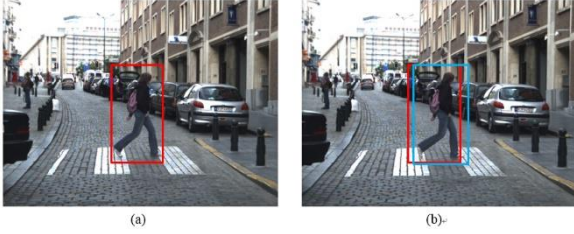
Fig.8 Sample of tracking a pedestrian in two consecutive images, red rectangle in (a) represents a found pedestrian and in (b) is the same position with (a), and the blue rectangle is the new rectangle to be computed by Lucas-Kanade optical flow method.
