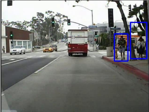
Fig. 23 Sample 5 of correctly classified pedestrians.
