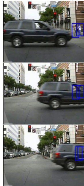
Fig. 25 Sample 1 of object occlusion and thus disturbance.
