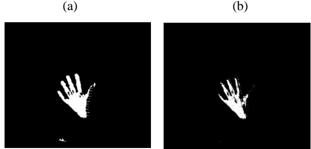
Figure 2. : (a) (b): Hand region segmented out by using depth image only and both depth image & skin color image. You can see from (a) that there is something in the same range as hand, so applying skin detection can avoid this problem.
