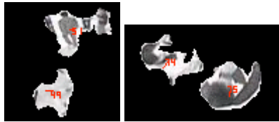
Fig. 9: Some edges in the image are too weak to complete the shape. (Number 49 & Number 74)
