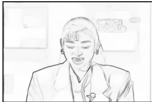
Figure 4. The gradient image obtained by the Sobel operator without grayscale reconstruction.
