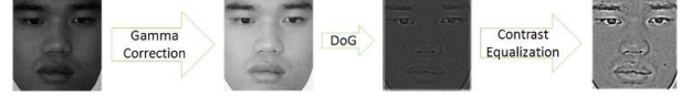
Fig. 6: Flowchart of illumination normalization by [16]. DoG operator generates abnormal lines on four sides of image due to Gaussian filter on the margin of image. We follow the recommendation of [16] to use constant padding when applying Gaussian filter. We can see that it generates abnormal lines (about 5 pixels in width) on four sides of image in Fig. 7. We do not want abnormal lines to influence the result so we remove them. After illumination normalization, we resize the image into 144 pixels in height and 128 pixels in width.
