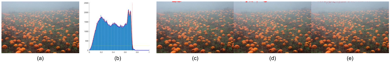
FIGURE 3. An example of applying histogram to the image to estimate the atmospheric light and the comparison results (a) Original image (b) Histogram. Atmospheric light estimation results using (c) DCP, (d) CAP, and (e) our proposed method (MCPA).
