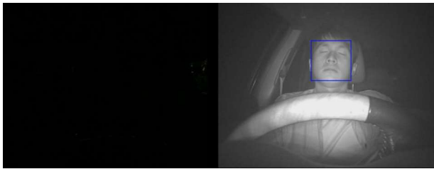
Fig. 7. The comparison between RGB camera (left) and IR camera (right) in the night.
