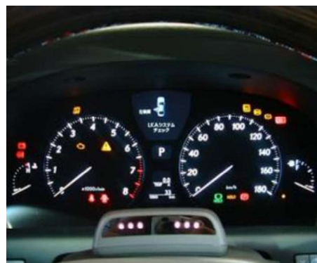
Fig. 1. The driver monitoring system on the LS 600h, and the red dot is infrared scanner [2].
