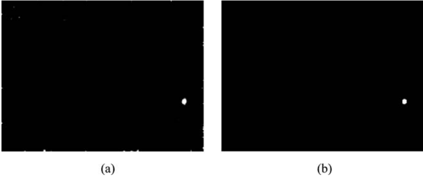
Fig. 7.12 (a) An image with many sparse spots. (b) Result of morphological operation based on 3 times of erosion operation and 3 times of dilation operation.
