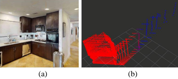
Fig. 5. The example of an accident assignment to the corridor. (a) Image of the kitchen with the corridor captured on the right-hand side. (b) Weighted point clouds.
