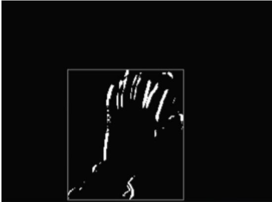
Fig. 2. D_i(x, y) with the threshold value 80 and bounding box.
