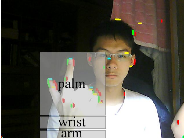
Fig. 13. Hand gesture is composed of palm, wrist, arm in the order top-down.
