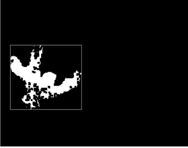
Fig. 5. Note that this image is taken in the dark environment. After mathematical morphology, the hand shape is stronger compared with its original.
