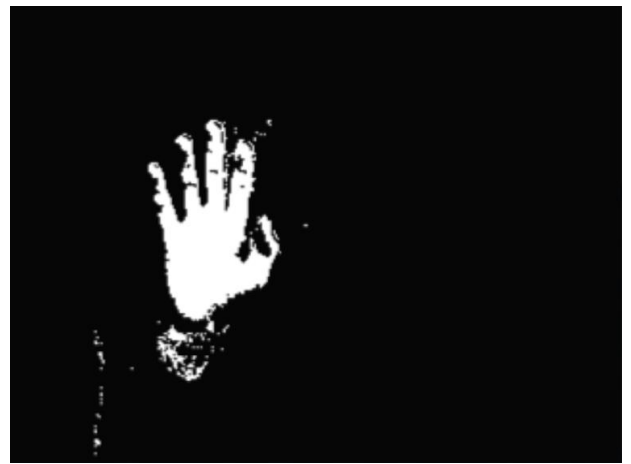
Fig. 4. The redundant information in skin color estimation image is removed by using the result of motion detection.
