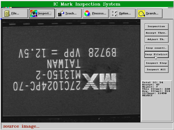
Fig. 14. The defective IC print mark with partial bad contrast.
