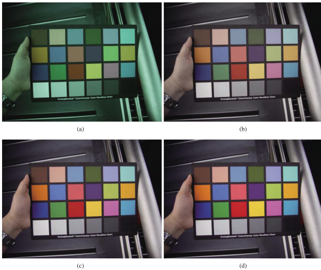
Fig. 6 (a) Unprocessed raw image from digital image sensor. (b) image is recovered after white balance by our method. (c) image is restored after color correction by our method. (d) image is restored by LSA
