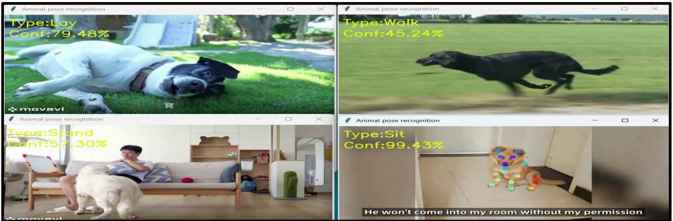
Figure 4: This image below showcases an "Animal pose recognition" system in action. It features four distinct panels, each displaying a dog in a different pose, along with the system's classification and confidence score: Top-Left: A dog lying on its back, identified as "Lay" with 79.48% confidence. Top-Right: A black dog in motion, identified as "Walk" with 45.24% confidence. Bottom-Left: A dog standing near a person on a couch, identified as "Stand" with 57.30% confidence. Bottom-Right: A dog sitting, identified as "Sit" with a high 99.43% confidence, and showing detected keypoints on its body.
