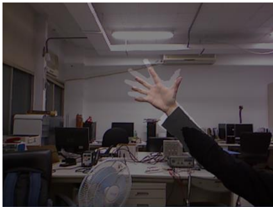
Fig. 1. Deviation in superposition for RGB and depth image.
