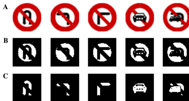
Fig. 12. Some examples of regulatory signs and their extracted object features. (A) The original road signs. (B) Their white object features. (C) Their black object features.
