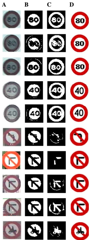
Fig. 15. Recognition results of real road sign patterns. (A) Test images captured by camcorder. (B) Corresponding white object feature of column (A). (C) Corresponding black object feature of column (A). (D) Their recognition results.
