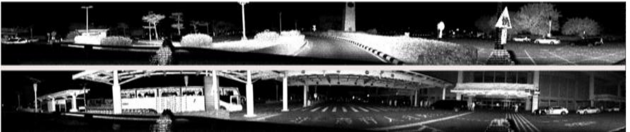
Figure 3.1 Images of point cloud data collected by Ouster OS-128 after coordinate transformation. Euclidean distance of each 3D point is represented by various intensity value. Note that the black image regions indicate the areas where the distances are undefined, such as the sky.
