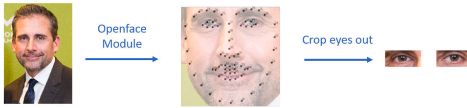
Fig. 2. Automated extraction of single eye images from a full-face photo using the OpenFace package. Key facial landmarks were identified (black dots in the center image) and then used to crop each eye for further evaluation.
