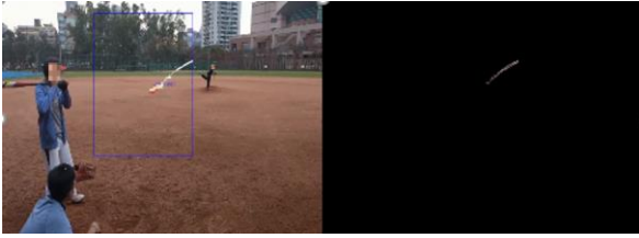
Figure 4: Ball detector: The blue area is the tracking area, and the color light path is the result of the optical flow algorithm.
