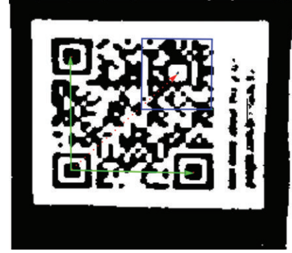
FIGURE 5: We extract blue rectangle to find the alignment pattern (radius = 30 pixels).
