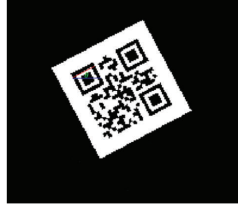
FIGURE 4: Red line is the width of finder pattern, and blue line is the estimated width.
