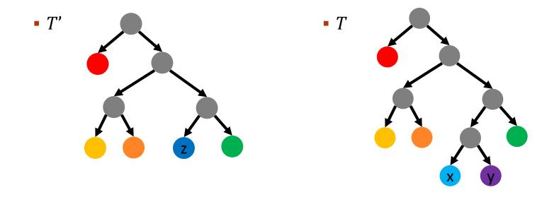
$B(T) = B(T') - \text{freq}(z)d_{T'}(z) + \text{freq}(x)d_{T}(x) + \text{freq}(y)d_{T}(y)$ =  $B(T') - (\text{freq}(x) + \text{freq}(y))d_{T'}(z) + \text{freq}(x)(1 + d_{T'}(z)) + \text{freq}(y)(1 + d_{T'}(z))$ = B(T') + freq(x) + freq(y)
