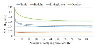
**Figure 6:** We show the relationship between the number of sampling directions and the accuracy of the recovered depth map, measured by the mean absolute error (in meter). Using more sampling directions could give more accurate results, at the cost of higher computational cost. We typically use 8 - 24 sampling directions per pixel.
