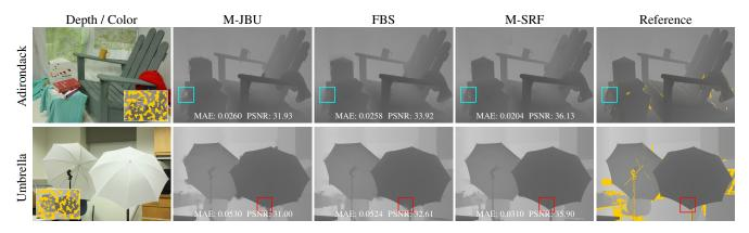
**Figure 12:** Comparisons of the Adirondack and Umbrella scenes in Middlebury 2014 data set [SHK\*14]. We allocate 20 milliseconds for M-JBU and M-SRF. The unoptimized FBS takes about 1.2 to 2.0 seconds. Our method can better preserve the depth discontinuities and achieve lower MAE and higher PSNR than M-JBU and FBS.
