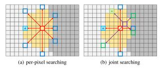
**Figure 3:** We sample lines to search for the representative pixels. (a) At each pixel with an invalid depth value (marked yellow), we uniformly sample a few directions for searching the best representative based on a similarity measurement. In this case, the neighbor labeled with a light blue asterisk is selected. (b) We stratify the sampling directions of adjacent pixels to search for different directions.
