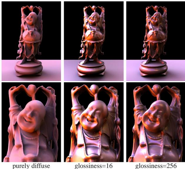
**Fig. 9** Material editing of a glossy *Buddha* in *Grace Cathedral*. The *Buddha* model is rendered using Phong model with different glossiness numbers. The bottom row shows closeup views of the top row. Our system allows changing parameters of BRDFs by sampling new BRDFs on the fly in a few seconds.
