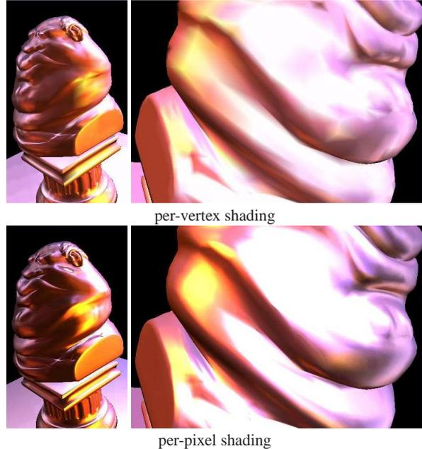
**Fig. 5** Comparisons between per-vertex shading and per-pixel shading. The left column shows rendering of a statue model with different shading methods. Closeup renderings of the same model from other view are shown on the right. Per-pixel shading clearly yields substantial improvement over per-vertex shading.
