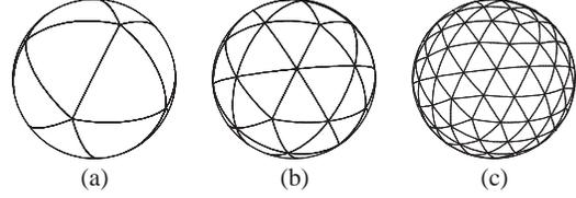
**Fig. 2** Geodesic sphere construction. Starting with the icosahedron ((a) subdivision level 0), successive levels (b,c) are generated by subdividing triangles into four sub-triangles, accomplished by adding geodesic edges connecting midpoints of original edges.
