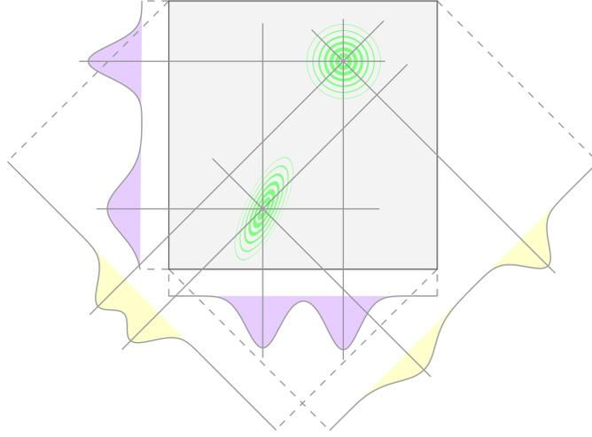
**Figure 5.2:** The green concentric rings depict a possible bimodal weighting function. The curves around the image indicate the convolved projections resulting from sweeping horizontal, vertical, and left and right diagonal Gaussian stripes across the screen independently. The horizontal and vertical sweeps alone (purple) are insufficient to determine the mode positions, but by adding additional diagonal sweeps (yellow) the correct modes can be determined.
