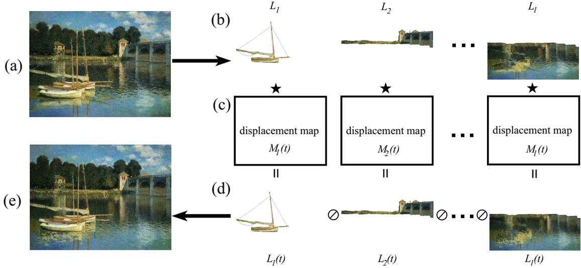
**Figure 6.1:** Overview of our system. The input still image (a) is manually segmented into several layers (b). Each layer  $L_i$  is then animated with a different stochastic motion texture  $M_i(t)$  (c). Finally, the animated layers  $L_i(t)$  (d) are composited back together to produce the final animation  $I(t)$  (e). The input painting is Claude Monet’s *The Bridge at Argenteuil*.
