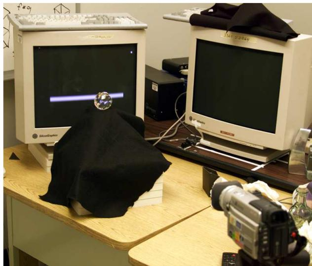
**Figure 5.5:** A photograph of our experimental setup for acquiring high accuracy environment mattes.
