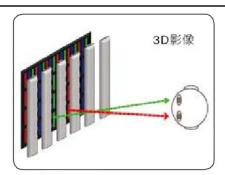
LC barrier could switch between 2D and 3D display modes.
