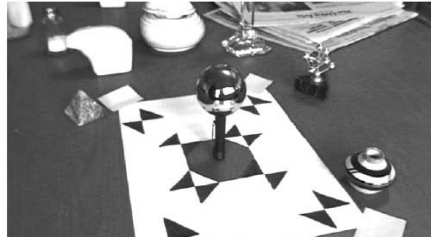
(b) Camera calibration grid and light probe
