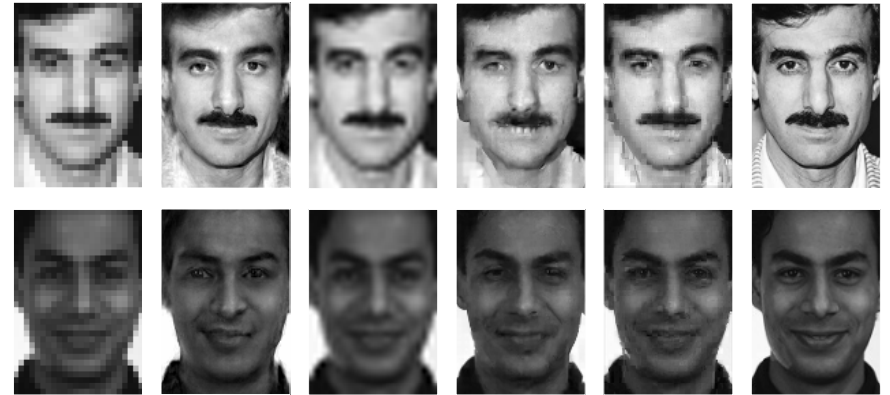
(a) Input low 24 \times 32 (b) Our results (c) Cubic B-Spline (d) Freeman et al. (e) Baker et al. (f) Original high 96 \times 128
