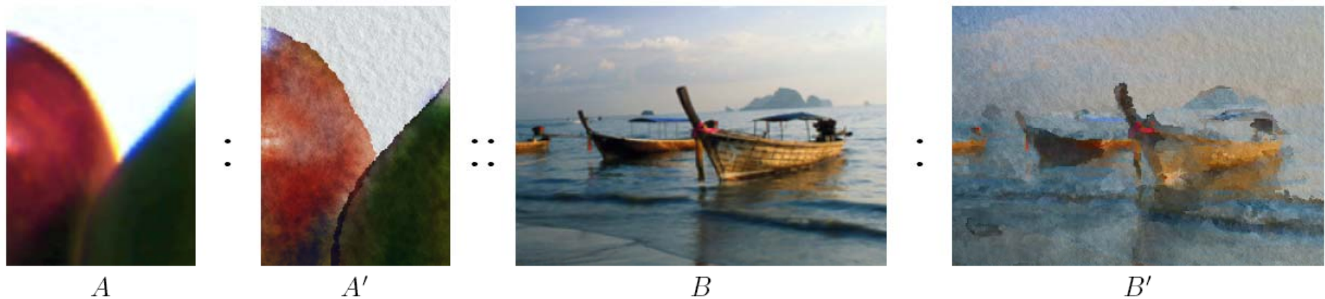
Figure 1 An image analogy. Our problem is to compute a new “analogous” image B' that relates to B in “the same way” as A' relates to A . Here, A , A' , and B are inputs to our algorithm, and B' is the output. The full-size images are shown in Figures 10 and 11.
