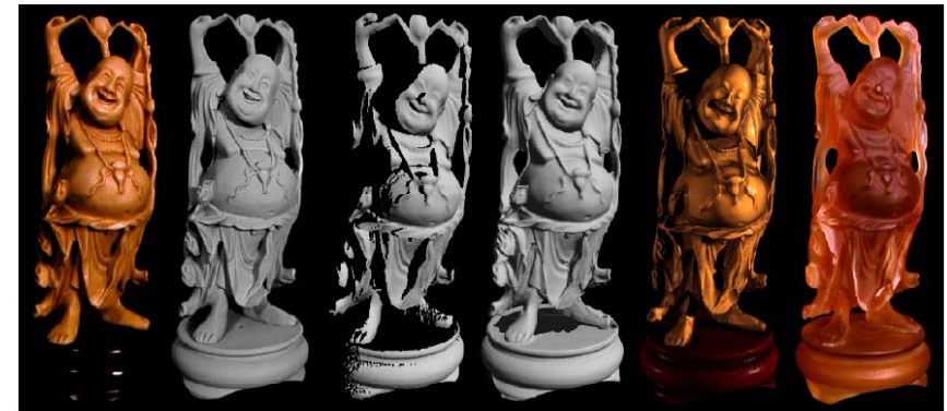
Photograph of original model Photograph of painted original Range surface from one scan Reconstruction before hole-filling Reconstruction after hole-filling Hardcopy
