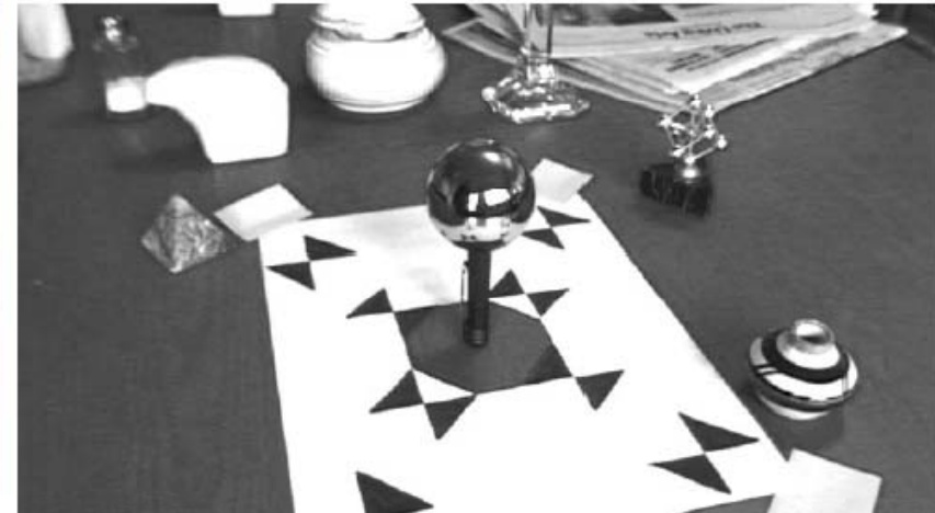
(b) Camera calibration grid and light probe
