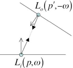
• Need to solve for L (only one unknown)  $L(p,\omega_o) = L_e(p,\omega_o) + \int_{S^2} f_r(p,\omega_o,\omega_i) L(t(p,\omega_i),-\omega_i) |\cos\theta_i| d\omega_i$
