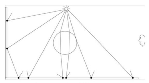
For 100 photons emitted from 100W source, each photon initially carries 1W.
