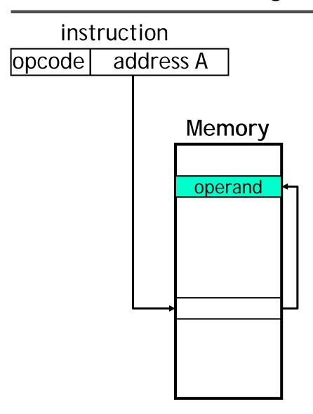
Address field contains the address of a pointer to the operand
