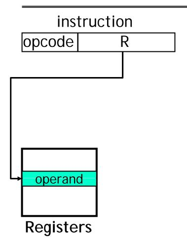
Address field contains the address of a register
