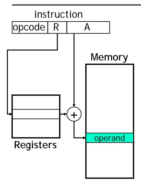
Address field could contain a register address and an address
