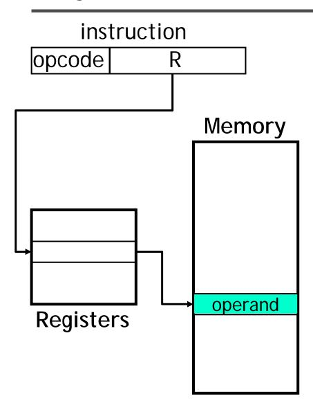
Address field contains the address of the register containing a pointer to the operand
