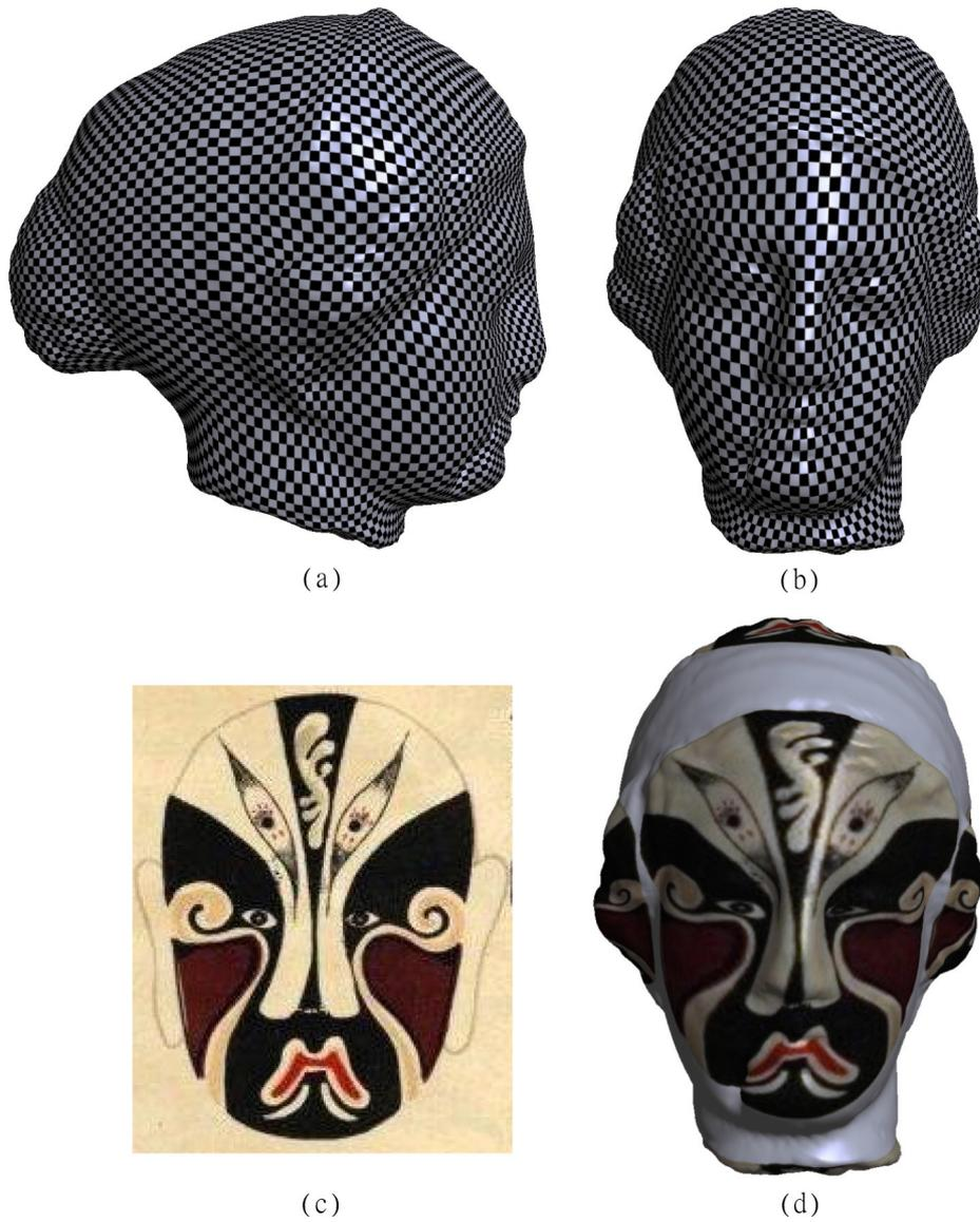
Texture mapping on the Igea's head. (a,b) The checkerboard texture mapping. (c) The 2D facial makeup in Chinese opera. (d) The facial makeup mapping on the Igea's head.
