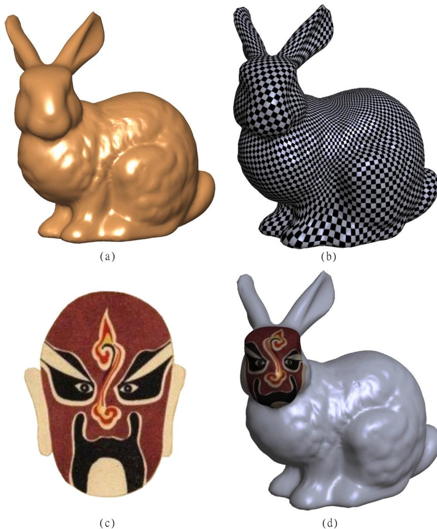
(a) The model surface  $M$  by the smooth algorithm. (b) The checkerboard texture mapping on  $M$ . (c) The 2D facial makeup in Chinese opera. (d) The facial texture mapping on  $M$ .
