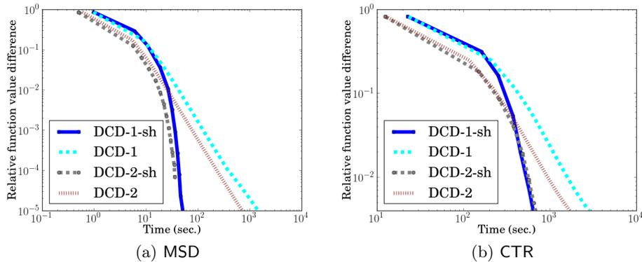
Figure 3: A comparison between two DCD algorithms. We present training time and relative difference to the dual optimal function values. L1-loss SVR with  $C = 1$  and  $\epsilon = 0.1$  is used. Data instances are normalized to unit vectors. DCD-1-sh and DCD-2-sh are DCD-1 and DCD-2 with shrinking, respectively. Both  $x$ -axis and  $y$ -axis are in log scale.
