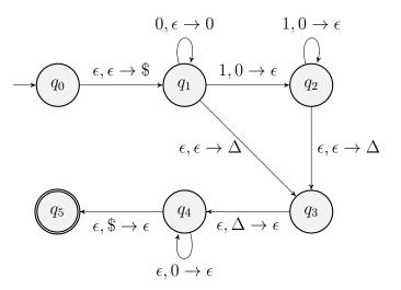
States  $q_0$ ,  $q_4$  and  $q_5$  are used to satisfy the first and the second conditions: single accept state and empty stack before accepting. Note that when adding  $q_4$  (which corresponds to  $q_{pop}$  in the slide), additional  $\epsilon \to \epsilon$  link would be generated, so we need  $q_3$  to satisfy the third condition: either push or pop in each transition.
