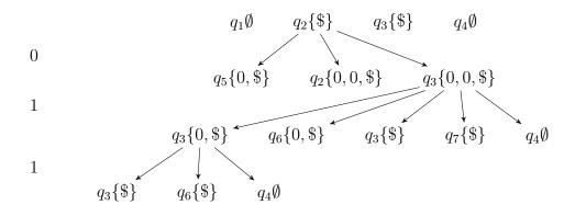
After processing the last input character, there's a branch stopping at  $q_4$ , so "011" is accepted. Common mistake: You cannot just show the path that leads to the acceptance or rejection. **Problem 3** (15 pts). Consider the following PDA P with  $\Sigma = \{0, 1\}$  and  $\Gamma = \{0\}$ :
