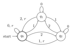
$\Sigma = \{r, 0, 1, 2\}$  and we treat r as a single symbol. Transform it to a GNFA and then obtain a regular expression by sequentially removing state  $q_2$ ,  $q_1$ , and  $q_0$ .
