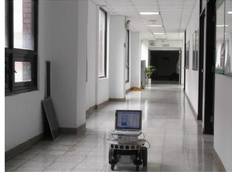
Fig. 1. The NTU-PAL5 robot with a SICK LMS291 laser scanner was used to verify the proposed approach in a long corridor.
