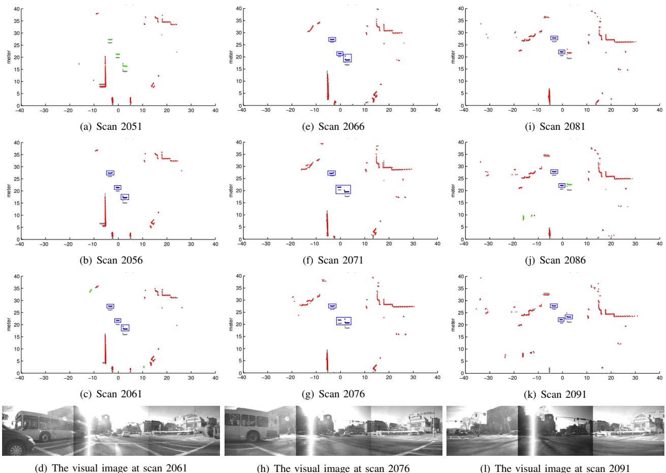
Fig. 4. MM-RANSAC results from scan 2051 to scan 2091. In these figures, grey dots are reference models, red dots are static objects, green dots are unknown objects, and blue dots and rectangles show moving objects.
