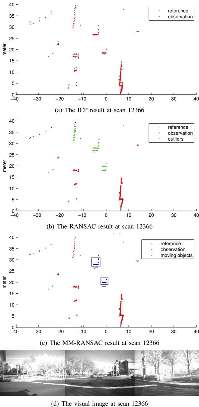
Fig. 2. Ego-motion estimation results in which the environments seen by the laser scanner is highly dynamic
