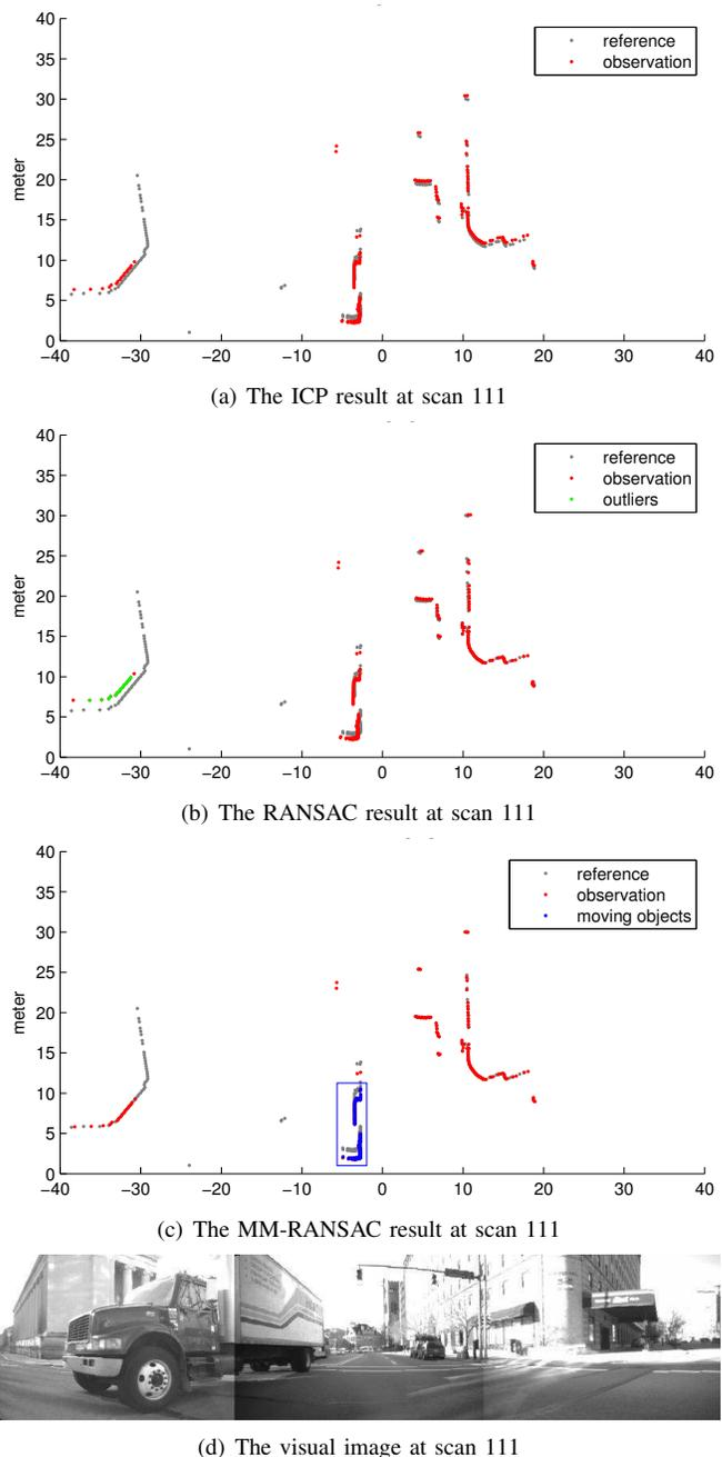
Fig. 1. Ego-motion estimation results in which the environments seen by the laser scanner is dominated by moving objects
