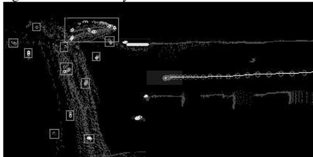
**Figure 4: Sick scanner range data processing, showing detected moving and fixed objects and vehicle trajectory**
