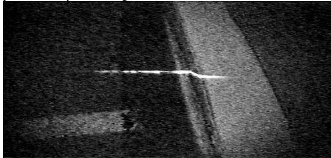
**Figure 2: Curb detection with light stripe sensor. The filtering and shuttering reduce the background illumination while leaving the infrared light stripe clearly visible. The shape of the stripe shows the contour of the street, curb, and sidewalk.**
