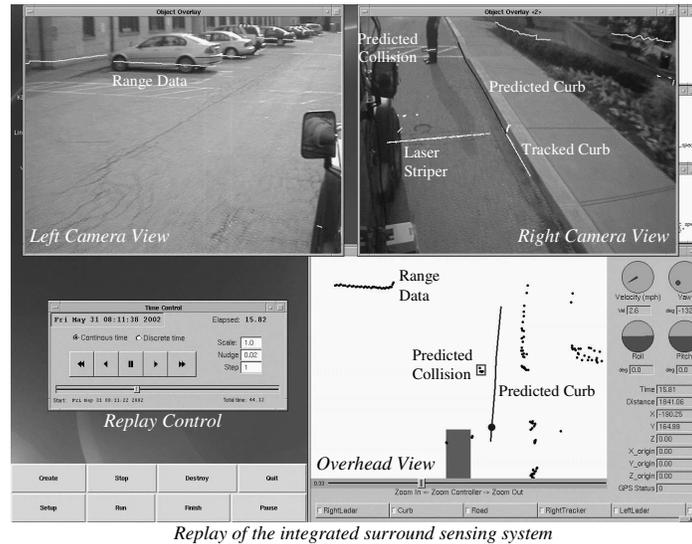
**Figure 8: Integrated Warning system: left camera view with overlaid range data; right camera view with overlaid range data and curb location; and fused map.**
