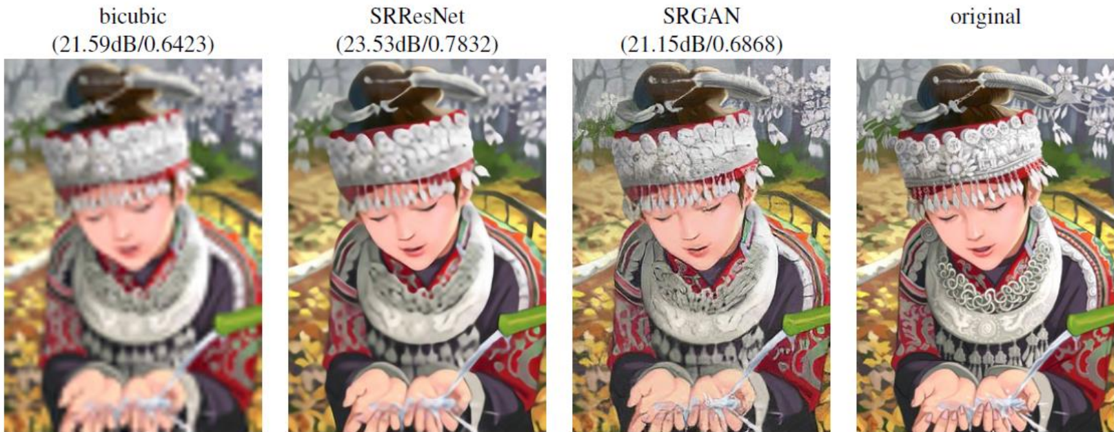
Figure 2: From left to right: bicubic interpolation, deep residual network optimized for MSE, deep residual generative adversarial network optimized for a loss more sensitive to human perception, original HR image. Corresponding PSNR and SSIM are shown in brackets. [4× upscaling]
