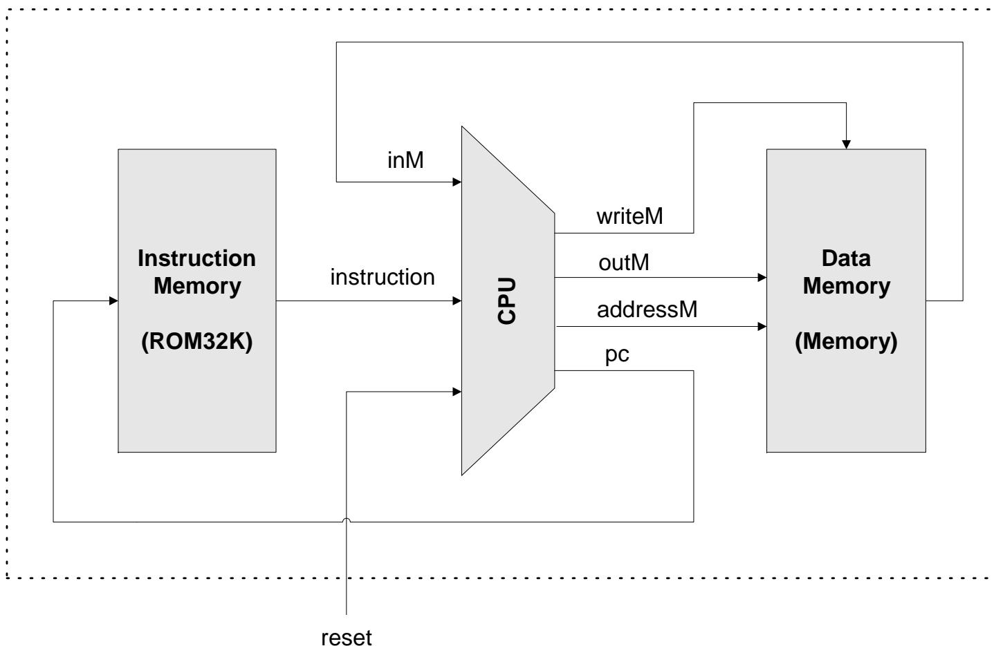
Both memory chips are 16-bit wide and have 15-bit address space.
