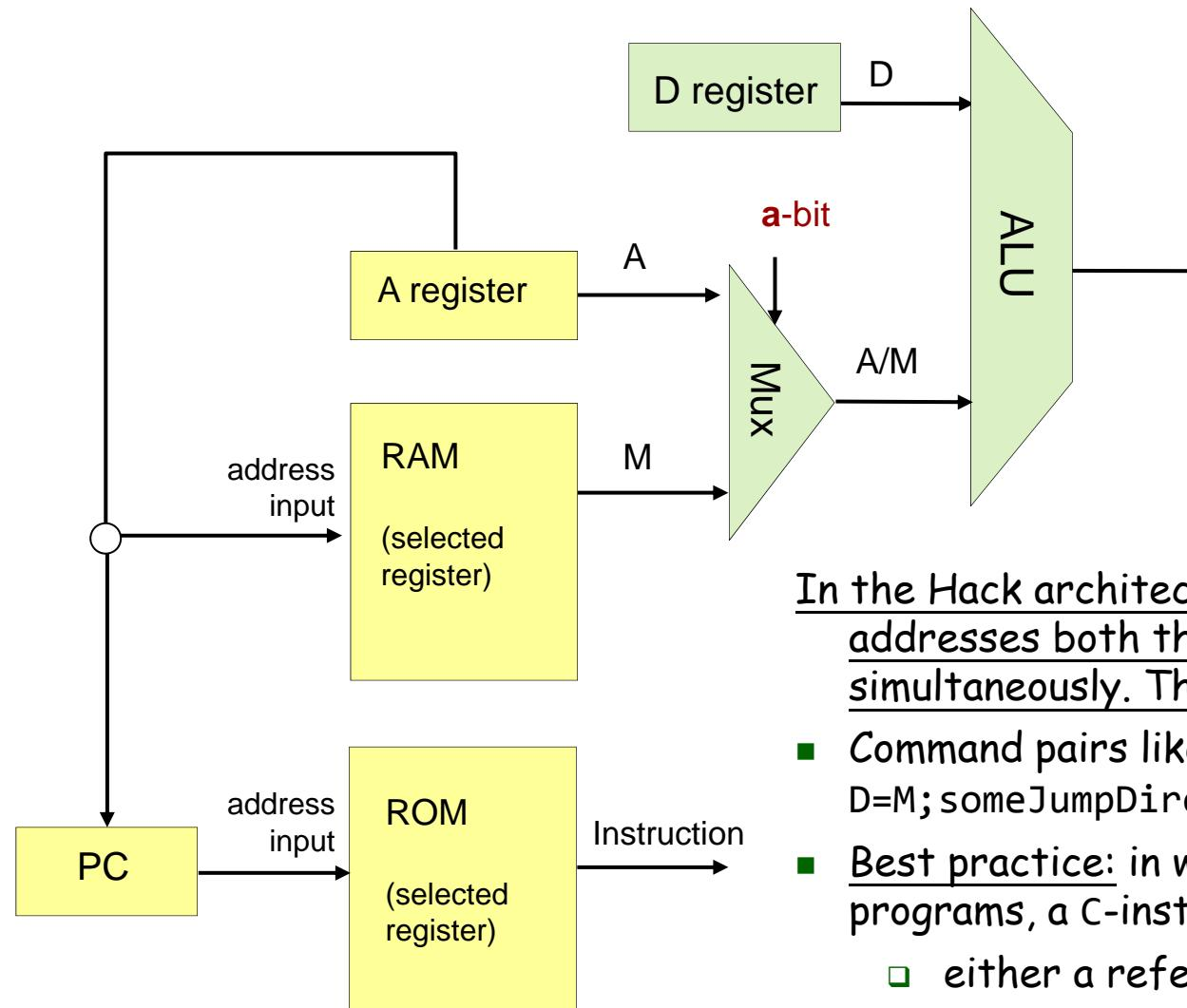
In the Hack architecture, the A register addresses both the RAM and the ROM, simultaneously. Therefore:
